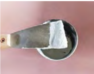
5. The final consistency should be like putty plasterboard.
