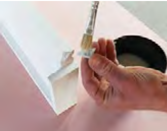
8. Liquid adhesive is applied to both parts.
